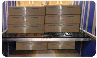
When used as a decking board, the cargo carrying capacity is determined by the beams supporting it.
