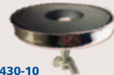
50430-10 Magnetic Flag Holder Secure warning flags with 2.3" diameter ceramic magnet rated at 80-lb. pull force. Holder has center screw and wing nut for flag attachment. Nylon insert prevents wing nut from backing off during transport.
