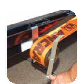
50391-10 Premium Cargo Strap Winder Constructed of zinc-plated steel for maximum durability, the new Strap Winder quickly assists in winding winch straps into rolls for storage. Designed to clip into trailer stake pocket or side rail. Weight: 2.7 lb./1.2 kg.
